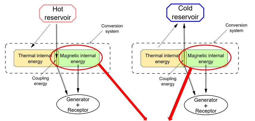
No matter how the temperature varies, <u>the harvested energy</u> is from **the coupling energy** and **internal magnetic energy**.
