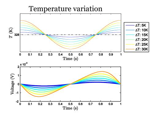
The generated voltage is proportional to temperature variation  $\Delta T = T_{max} - T_{min}$
