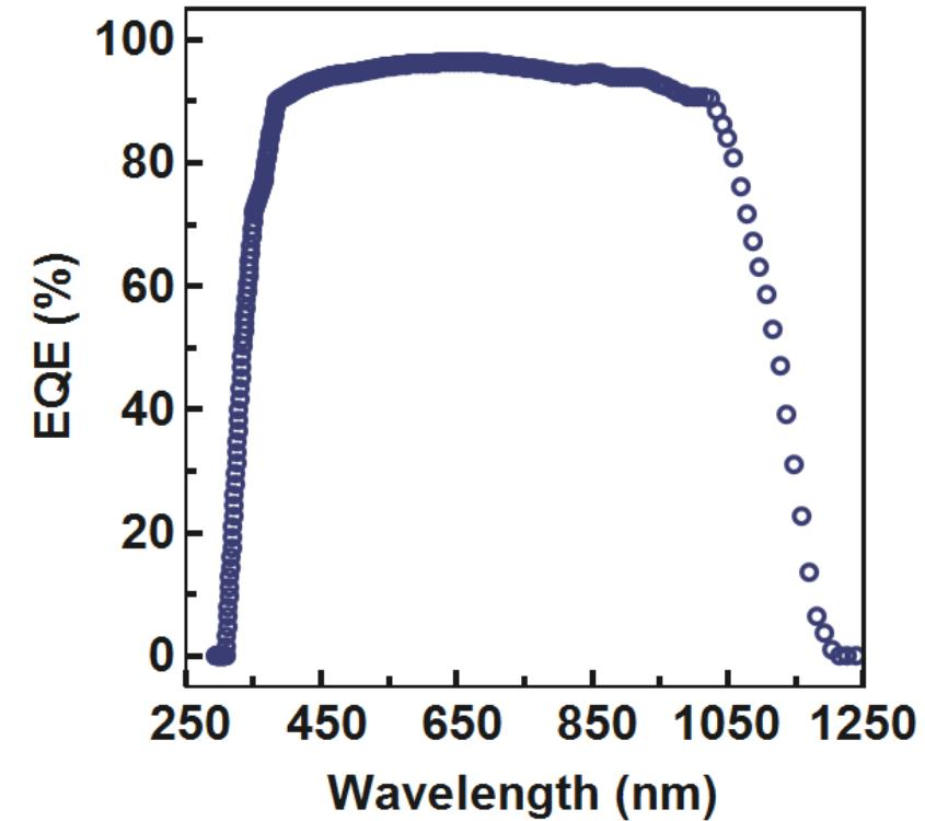
SunPower C60® mono-crystalline silicon solar
