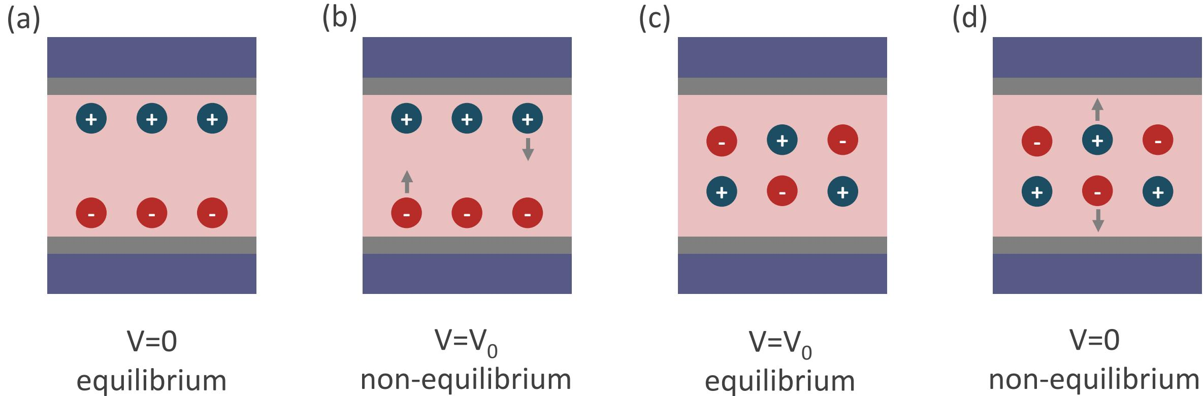
Going from (d) to (a): mobile ions drift towards the interfaces to screen the built-in electric field.
