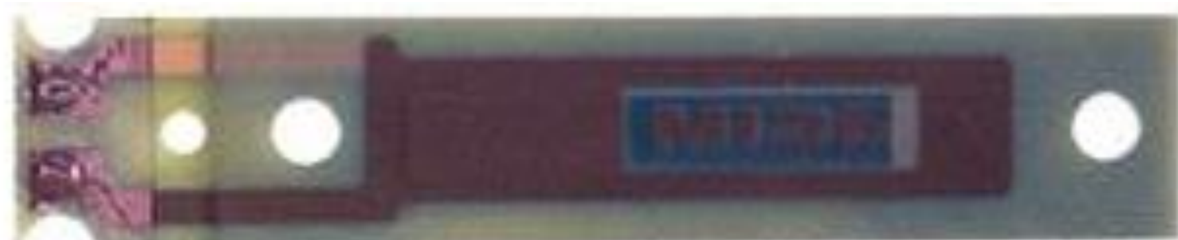
Figure 1. PPA-1022 PZT transducer [2]
