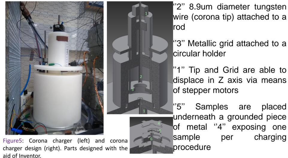
Figure5: Corona charger (left) and corona charger design (right). Parts designed with the aid of Inventor.
