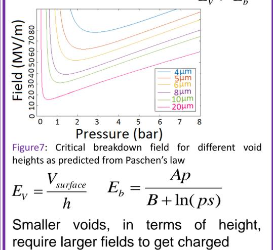
Figure7: Critical breakdown field for different void heights as predicted from Paschen's law
