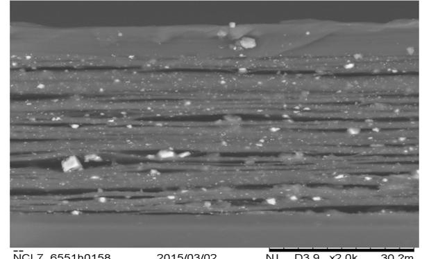
Figure1: Cross section of the virgin material with thickness of 80µm. Image taken with the aid of Scanning Electron Microscope TM3030
