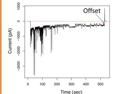
Figure8: Current flowing from the sample during charging process. Data obtained with the aid of Electrometer Keithley 6517b
