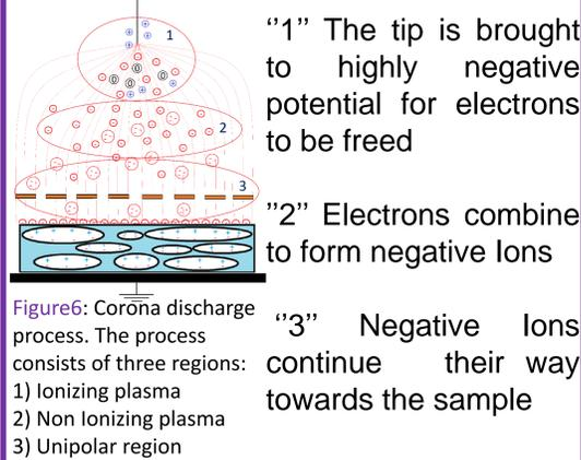
Figure6: Corona discharge process. The process consists of three regions: 1) Ionizing plasma 2) Non ionizing plasma 3) Unipolar region
