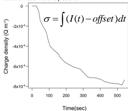
Figure9: Charge density obtained by integration of the current slope (figure 8)
