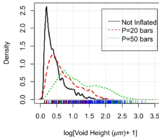
Figure3: Density of voids height distribution within the material for different inflations
