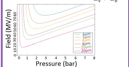
Figure7: Critical breakdown field for different void heights as predicted from Paschen's law
