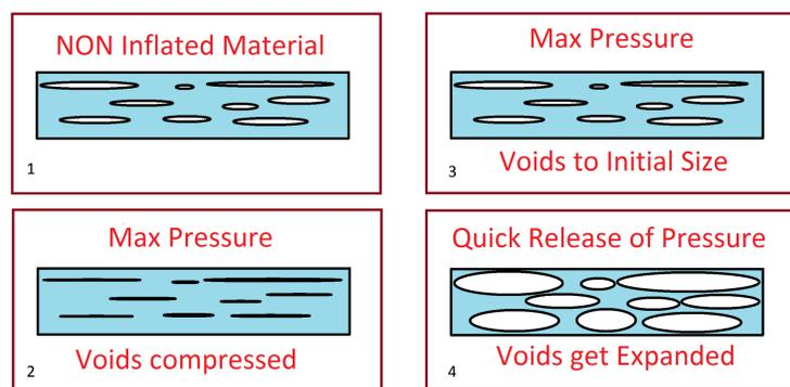
Figure2: Gas Diffusion Expansion (GDE) procedure. 1) Sample in its initial state 2) The voids get compressed 3) The pressure inside the voids gets equal to the external pressure 4) The voids get expanded
