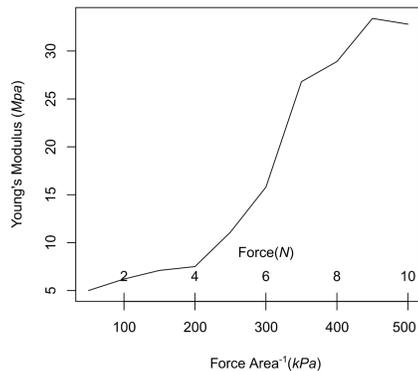
Figure11: Modulus of elasticity during compression at different loads. Data taken with the aid of Dynamic Mechanical Analyzer "DMA8000"
