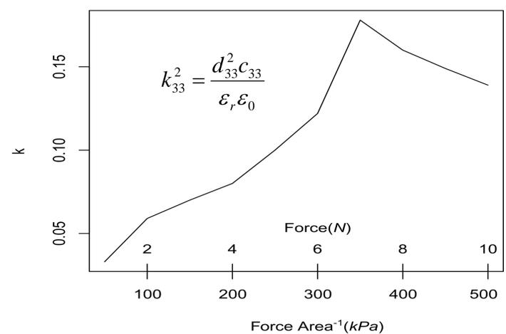
Figure12: Calculated k for different loads based on the data from figures 10 and 11
