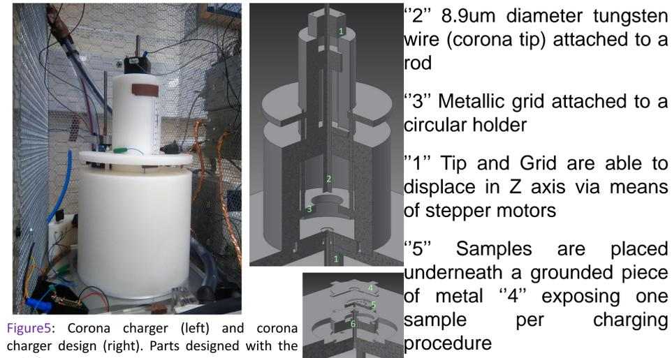
Figure5: Corona charger (left) and corona charger design (right). Parts designed with the aid of Inventor.
