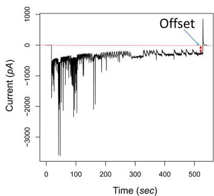
Figure8: Current flowing from the sample during charging process. Data obtained with the aid of Electrometer Keithley 6517b
