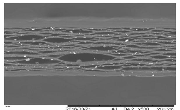
Figure4: Cross section of an inflated material. The inflation was done via GDE procedure with max pressure time of 20 minutes and pressure release of 1.5 minutes. Resultant thickness of 125µm. Image taken with the aid of Scanning Electron Microscope TM3030
