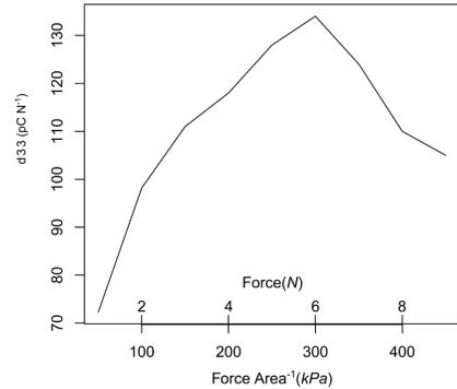
Figure10: Static  $d_{33}$  value measured at different loads. n=3
