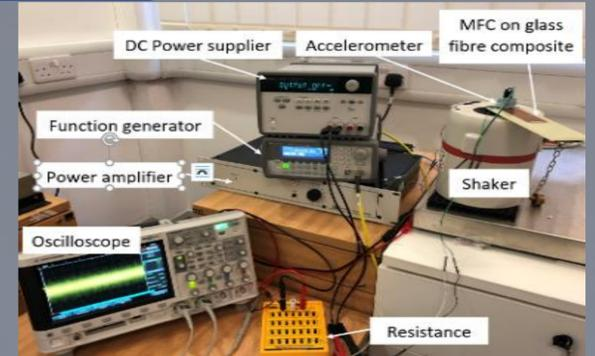
Figure 3. Experimental setup to characterise the harvester.
