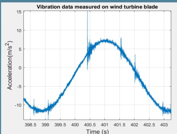
Figure 1. Practical vibration acceleration input on Z orientation.
