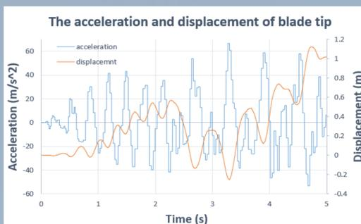
Figure 6. FEA result of wind turbine blade tip.
