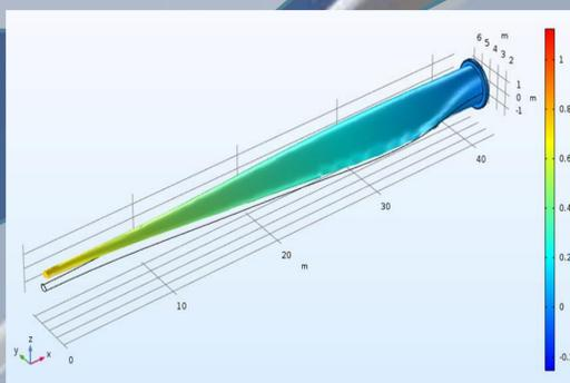
Figure 5. FEA model of turbine blades.
