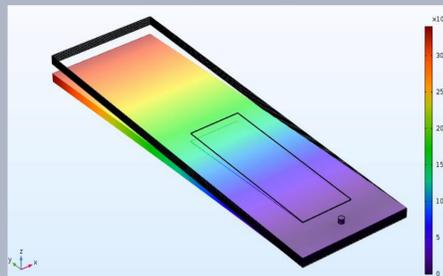
Figure 4. FEA model of glass fiber cantilever.
