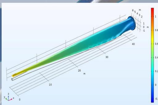
Figure 5. FEA model of turbine blades.
