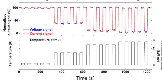
Figure 4 Signals change while light irradiated cyclically over time, self-powered by Seebeck voltage.
