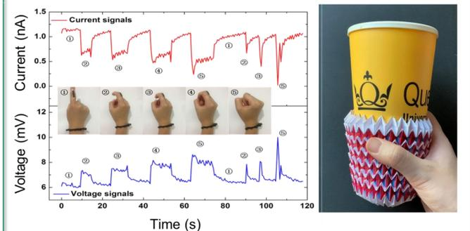
Figure 5 It as a self-powered wearable sensor for index finger positions, at  $\Delta T \sim 20 K$ . And it harvests secondary heat as a generator.
