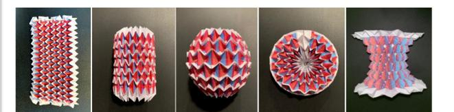
Figure 7 Demonstration of a 90-couples "magic ball" shape conformable TE device.
