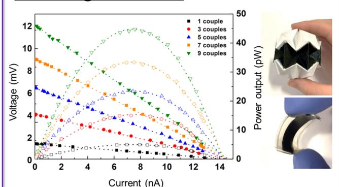
Figure 6 The power output (left) of 6-couples TE device under  $\Delta T \sim 20 K$ . Two different designs for TE device assembling (right).
