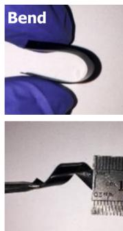
Figure 1 The tensile properties for self-standing PU/Na<sub>x</sub>(Ni-ett)<sub>n</sub> composites films. Optical pictures showing flexibility under bending and twisting.
