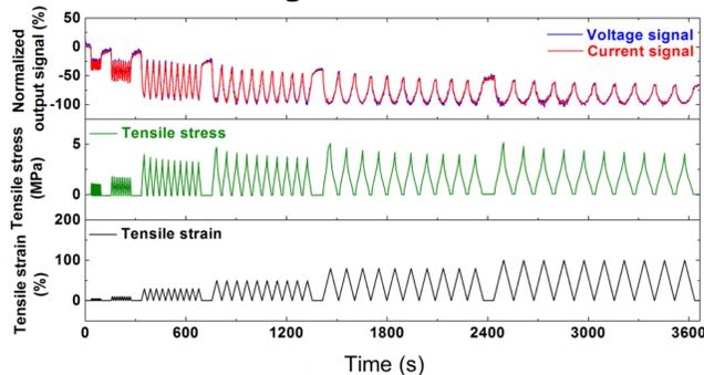
Figure 3 Signals change under cyclically tensile strain, self-powered by Seebeck voltage generated at  $\Delta T \sim 50K$ .
