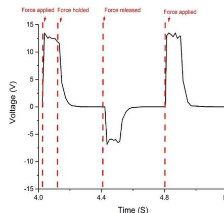
Figure 7: Energy output pulse of PDMS ferroelectret at the optimal resistance of 65 MΩ under 800N slow walking mode
