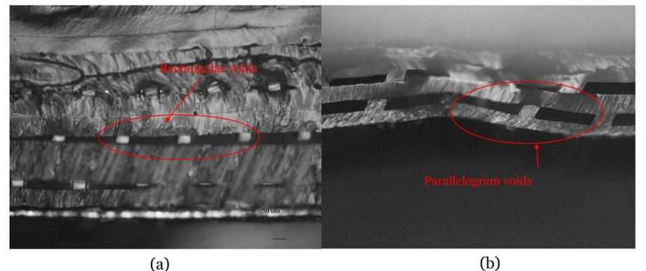
Figure 9: The image of the cross section image for multilayer PDMS ferroelectret (a) rectangular PDMS ferroelectret (b) parallelogram void PDMS ferroelectret
