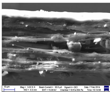
Figure 2: SEM photographs of cross sectional view of commercial ferroelectrets
