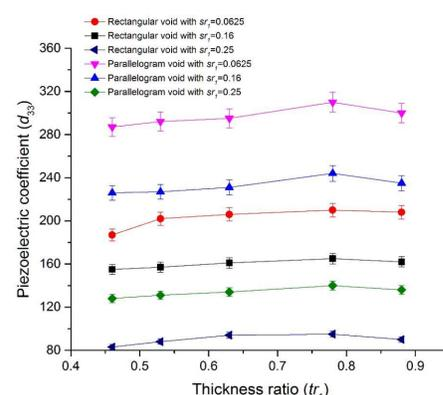
Figure 5: The measured piezoelectric coefficient varying with the thickness ratio for one void layer PDMS ferroelectret
