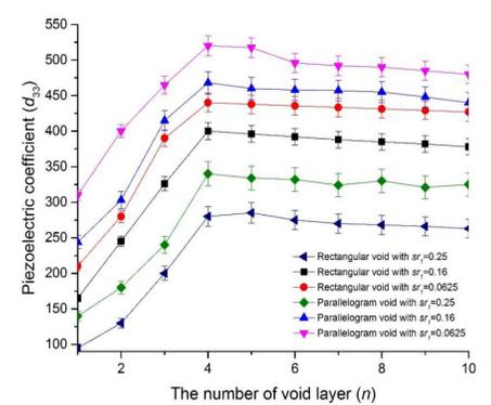
Figure 6: The measured piezoelectric coefficient varying with the number of void layers
