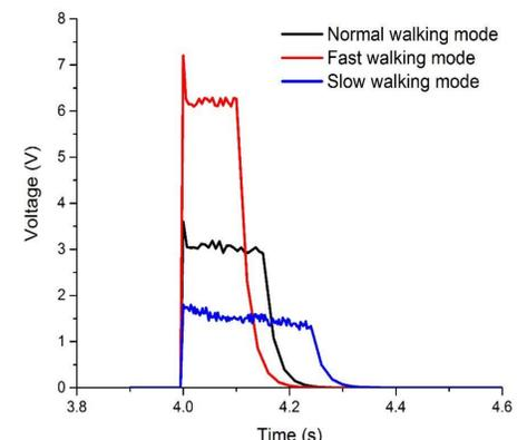
Figure 8: Output voltage pulse for three different walking mode at the resistance of 10 MΩ under a constant force of 800 N
