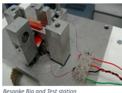
The single PZT beam could produced 9.55mJ of energy with a load of 470Kohms @ 3Hz. This gave a 0.3milliwatts average power figure.
