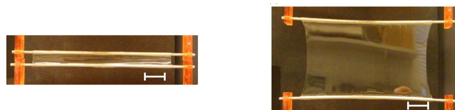
Figure 5: Membrane stretched under pure-shear conditions [5].
