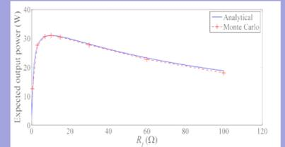
Figure 4: Expected power under broadband random vibration
