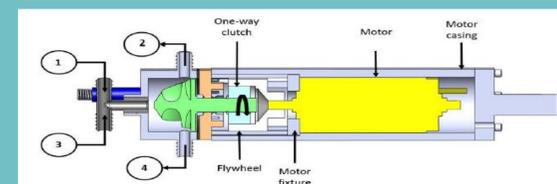
Figure 10: Cross section of Hydraulic Shock Absorber
