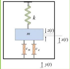
Figure 1: Schematic diagram of linear harvester
