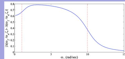
Figure 6: Correction of the expected output power of the simulated energy under band-limited excitation ( $\omega_1 = 1 \text{ rad/s}$  and  $\omega_2 = 10 \text{ rad/s}$ ) harvester versus  $\omega_n$
