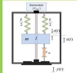
Figure 2: Schematic diagram of rotational harvester
