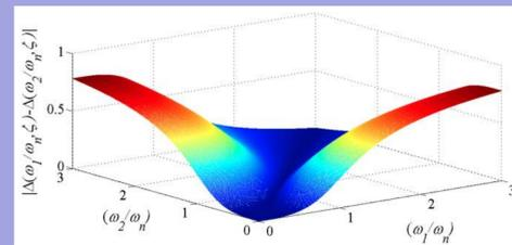
Figure 5: Correction factor for calculation of the expected output power of energy harvester under band-limited excitation for a device with  $\xi = 0.5$
