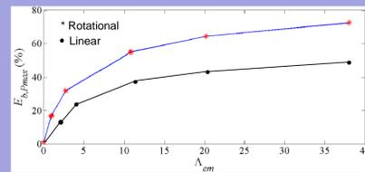
Figure 3: Efficiency of rotational/Linear electromagnetic energy harvester versus  $\Lambda_{em}$
