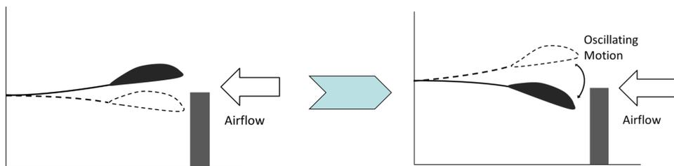
Figure 1. Operation principle of the flapping generator
