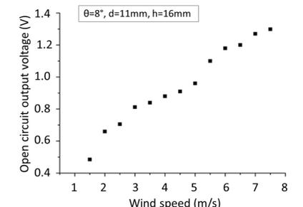
Figure 10. Open circuit output voltage in varying flow speed conditions with optimal configuration and load
