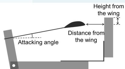
Figure 3. Mechanical structure design variables
