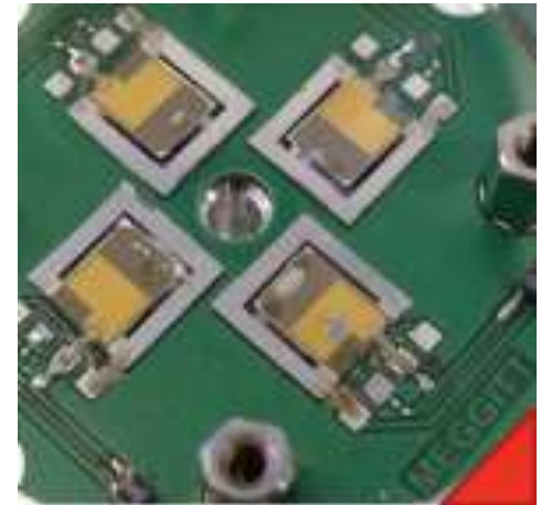
Up to 4 micro generators are combined (two are sufficient for the proper system functionality)
