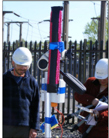
Fig. 1 Measuring magnetic flux density using voltage logger.
